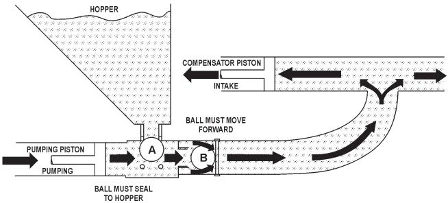
Figure 11. Pumping Pistons
